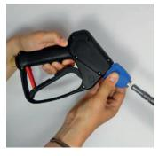
To change the lance, **release the trigger** and use the quick connection to swap.
