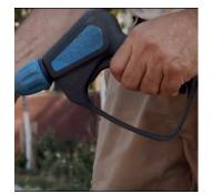
The boiler is only active when the trigger is pulled.
