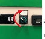
Keep trigger pressed until tower light comes on, which takes around 60 s. Light on = ready to use
