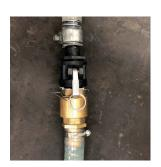
Connect the level sensor plug.
