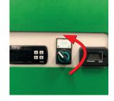
Optional step: Keep the trigger pressed to cool the boiler down. Wait until the temperature on the thermostat drops below 60°C / 140°F.
