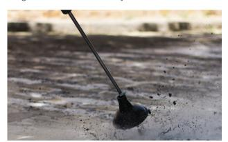
**PRESSURE LANCE:** This lance is our highest-pressure lance (20 bar). Despite being lower pressure than conventional 'high pressure' solutions, Foamstream achieves a more effective treatment result due to its prolonged high temperature delivered by an insulating foam blanket which reduces surface damage.
