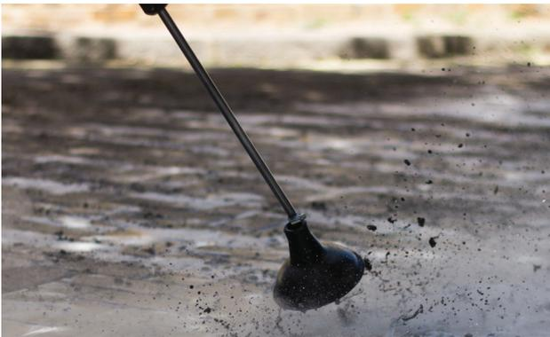
**PRESSURE WAND:** This wand is our highest-pressure wand (290psi). Despite being lower pressure than conventional 'high pressure' solutions, Foamstream achieves a more effective treatment result due to its prolonged high temperature delivered by an insulating foam blanket which reduces surface damage.
