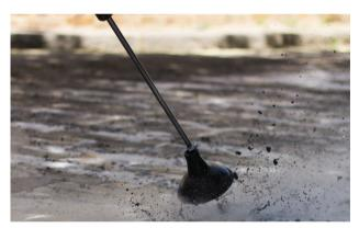
**PRESSURE WAND:** This wand is our highest-pressure wand (290psi). Despite being lower pressure than conventional 'high pressure' solutions, Foamstream achieves a more effective treatment result due to its prolonged high temperature delivered by an insulating foam blanket which reduces surface damage.
