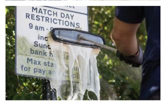
**NYLON SCRUB BRUSH:** A more traditional rectangular brush head, this wand is perfect for cleaning tasks such as removing moss, algae or debris from smooth metal or plastic surfaces such as signs and trash cans.
