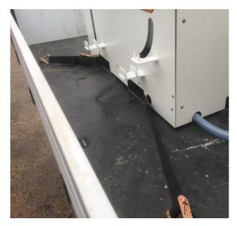
Figure 21 - Strapping of the M1200 to the vehicle
