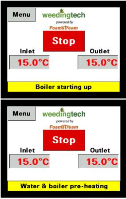
Figure 15 - Running screen of the PLC
