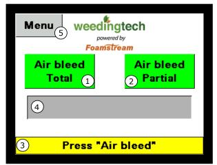
Figure 12 - Start-up screen of the PLC
