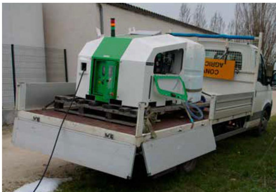
The Foamstream M1200 mounted on a flatbed truck
